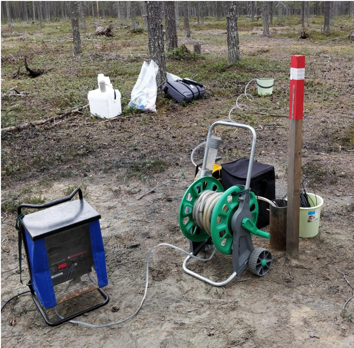
Figure 5. Grundfos BMI-MP1-230V pump flushing a well for the sample set B-10-17HYD017. May 2018.
