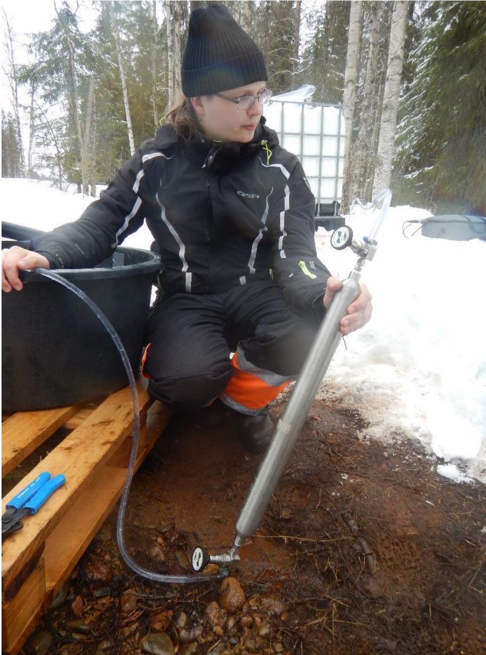
Figure 7. Collecting CFC-12 and SF 6 sample D-3-17MOS8193 in an aluminium container. Photo: Kirsti Korkka-Niemi, April 2018.
