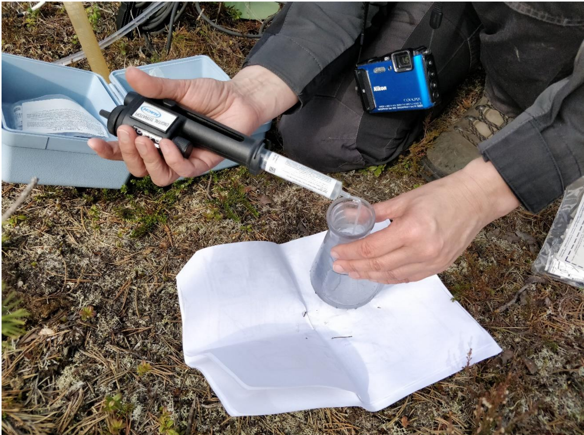
Figure 8. HACH titrator used to measure \text{CaCO}_3 content. May 2018.
