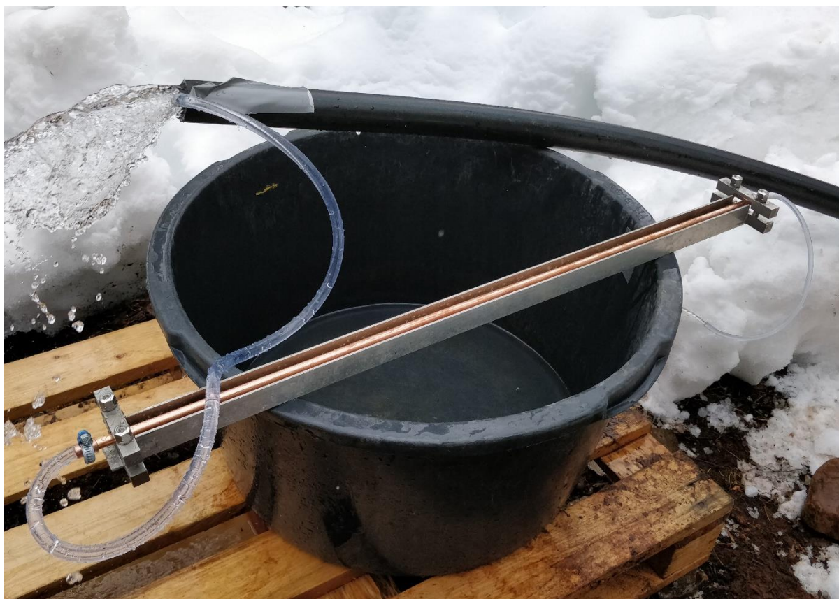
Figure 6. Copper tube used in sampling of the noble gases (D-3-17MOS8193). Photo: Kirsti Korkka-Niemi, April 2018.
