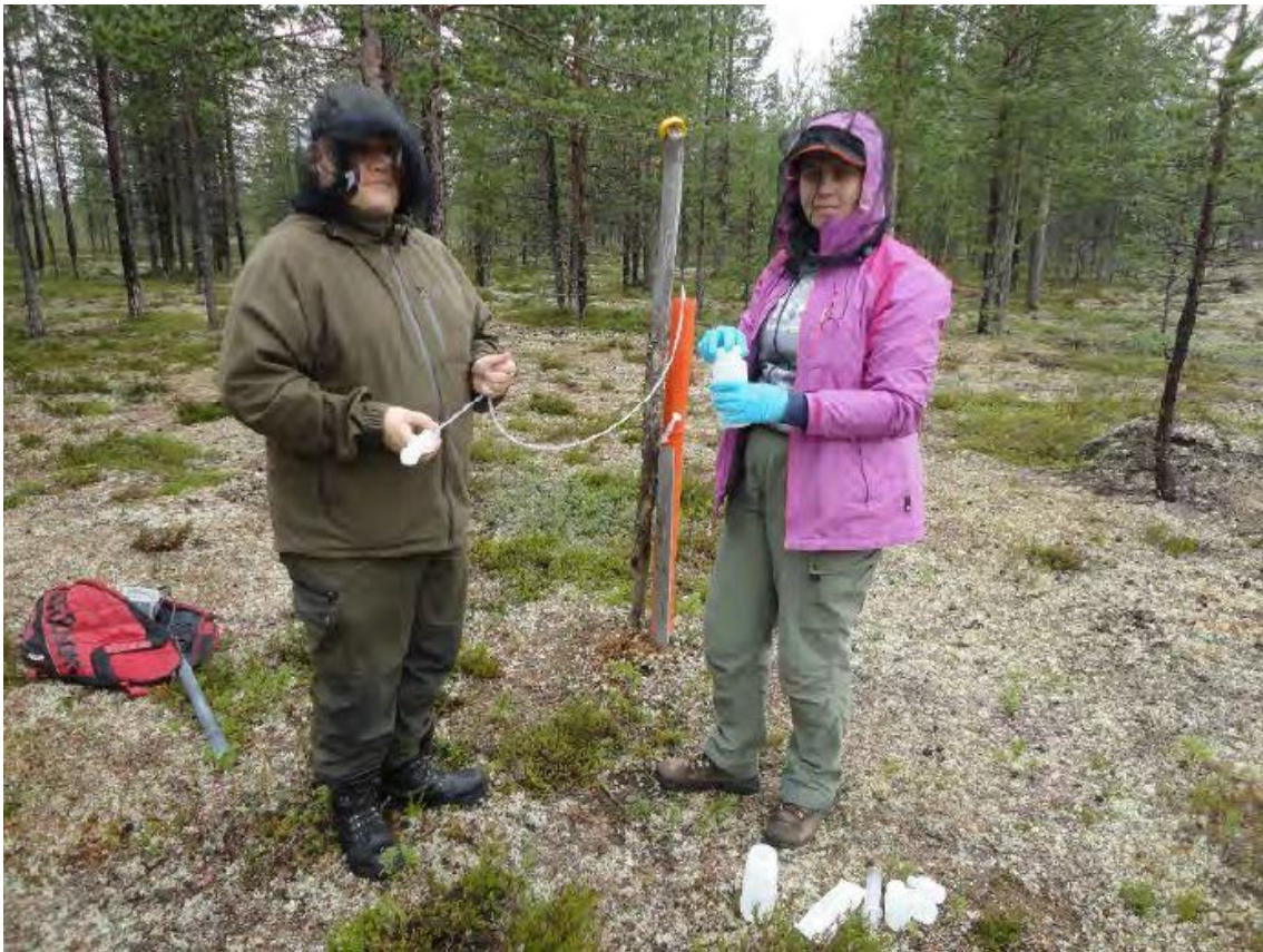
Figure 5. Groundwater sampling from a groundwater observation well using a minipiezometer and a syringe. Photo: Kirsti Korkka-Niemi.
