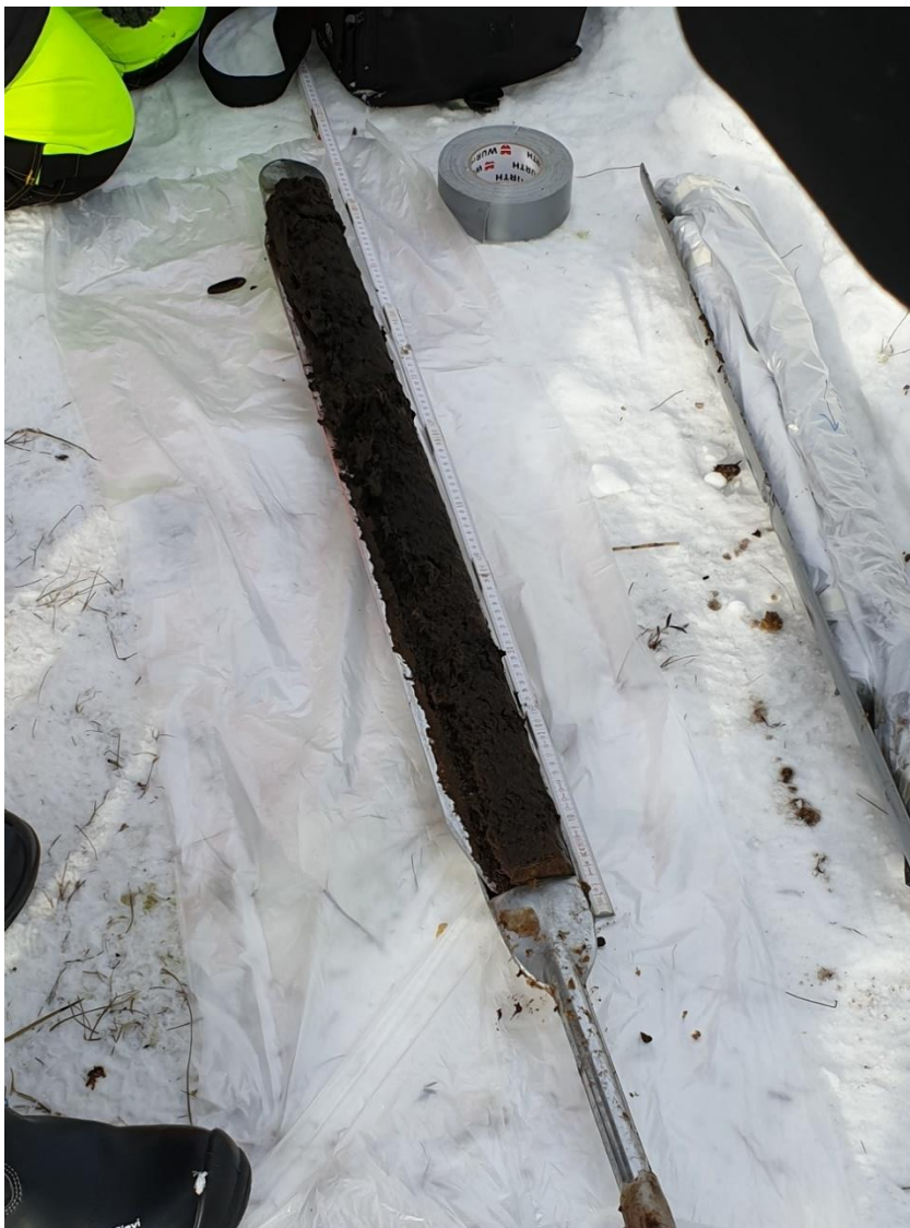
Figure 5: A Russian peat corer at sample site PEAT7 with the peat core exposed.
