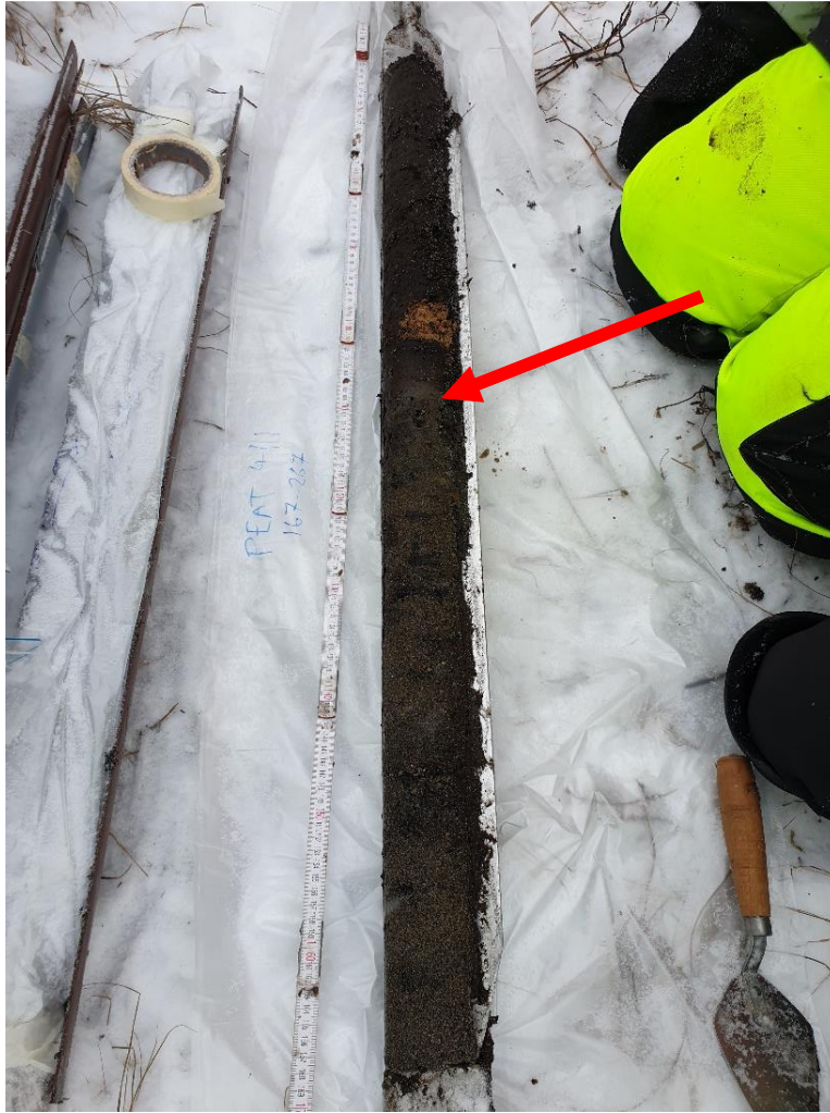
Figure 20: Peat core from sampling point PEAT4. The sudden change in composition from organic dominated to a mixture of clastic/organic is seen in the top side of the figure under the light brown unit, which is decomposed woody material.
