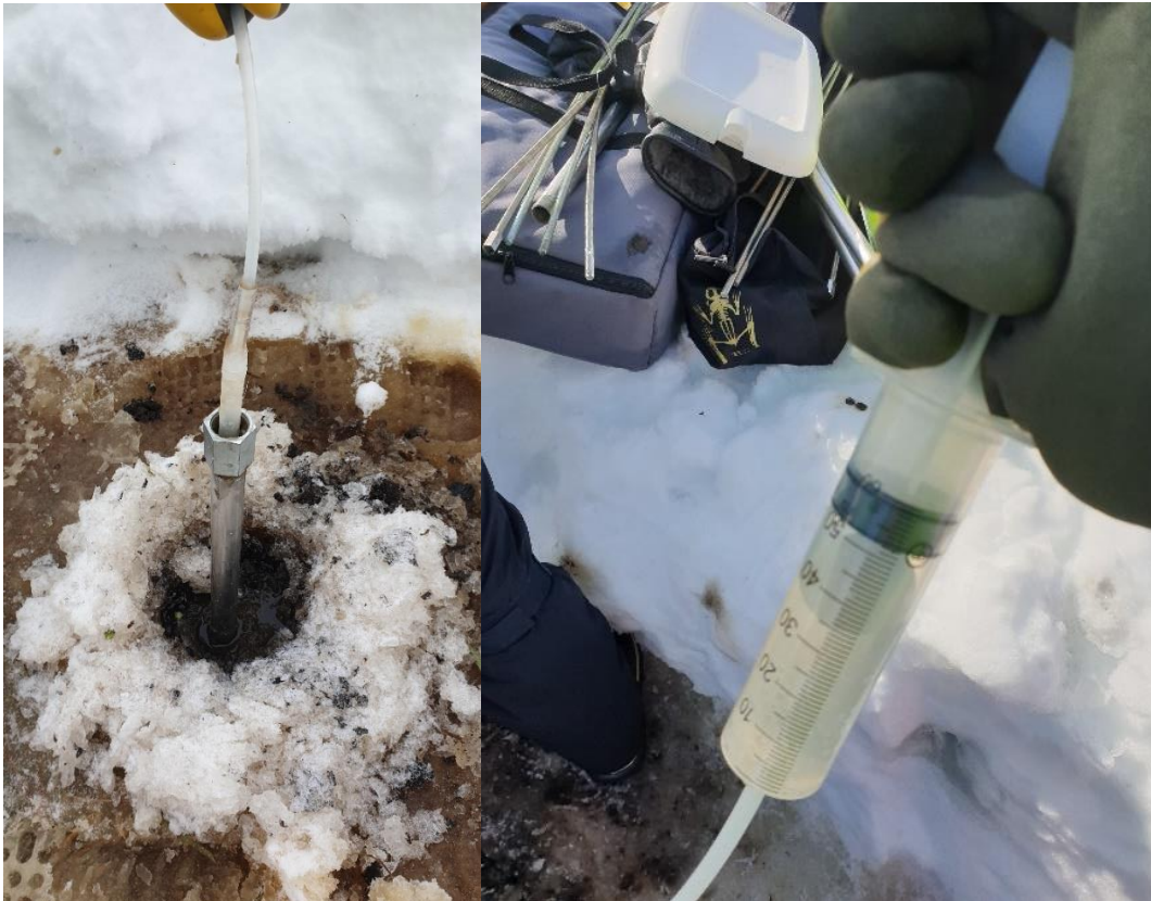
Figure 8: Mini-piezometer is inserted into the cover tube, stage 3 of the procedure. Afterwards, the sample is drawn using a syringe.
