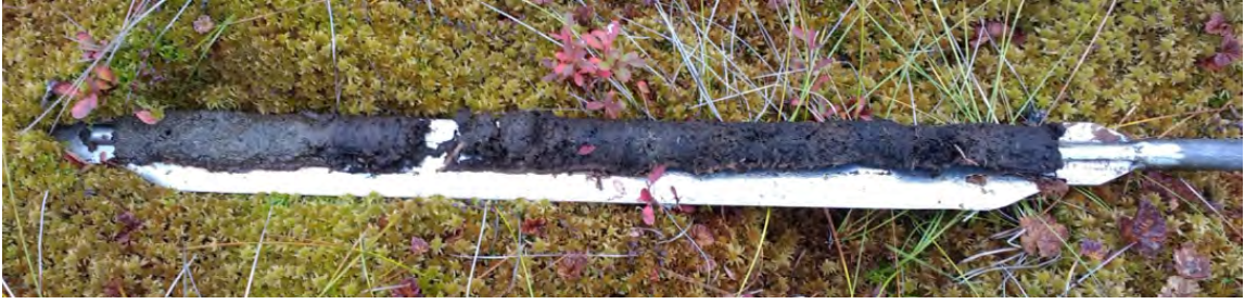
Figure 5. Russian peat corer with a sample of peat and underlying sediment at the eastern part of Porokodanjänkä mire. Photo by Markus Valkama.
