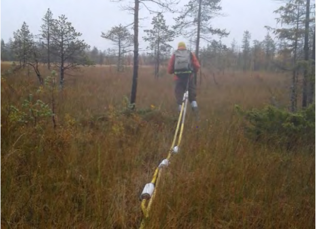
Figure 6. GPR acquisition with the 50 MHz and 100 MHz antennas at the west basin of Porokodanjänkä mire. Photo by Emilia Koivisto.
